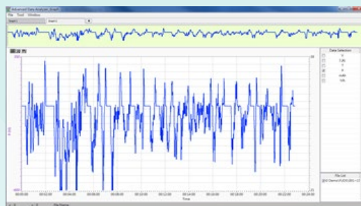
▲ FUDS Cycle Test Figure Obtained Using MCL2 Series
